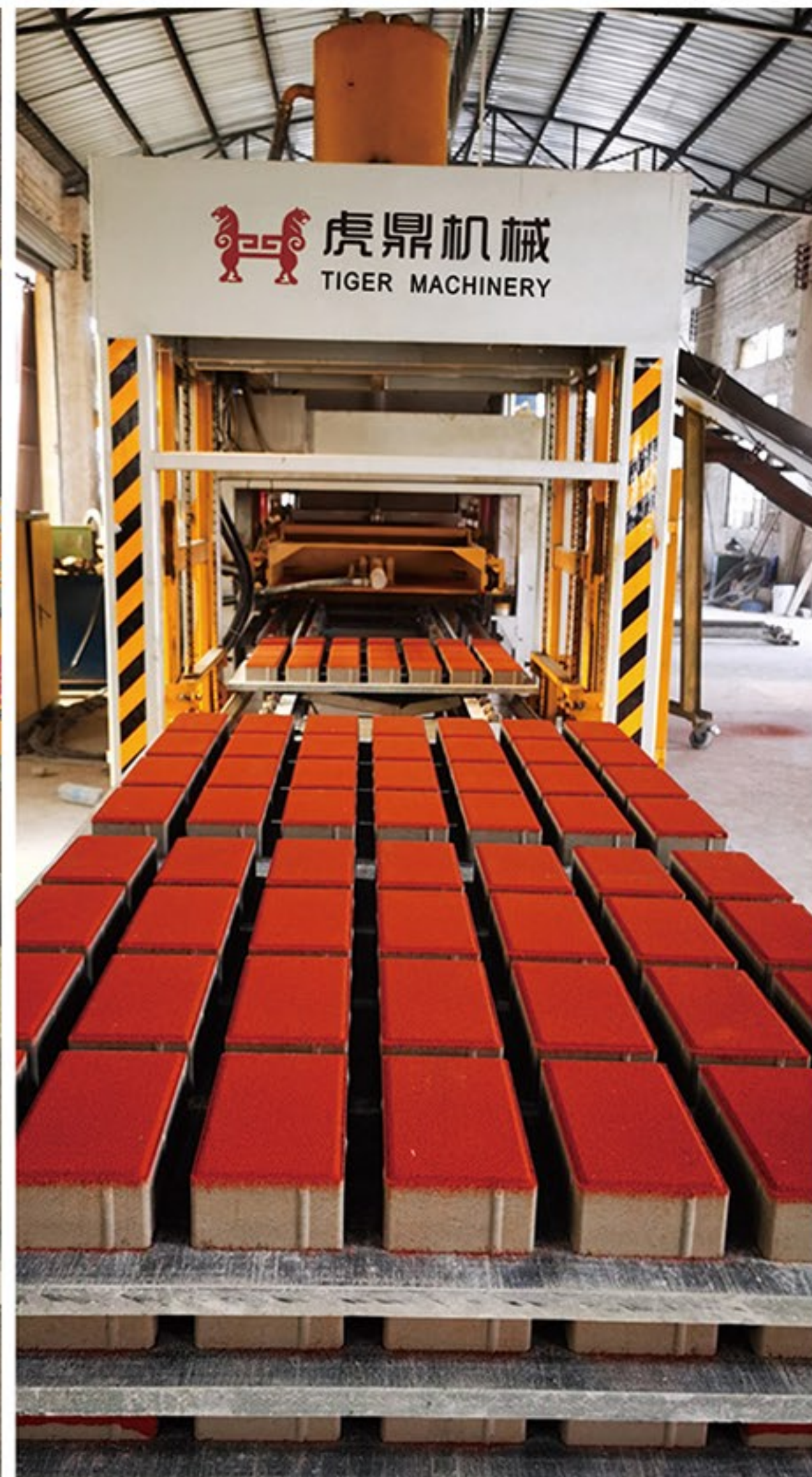
Production of paving blocks
