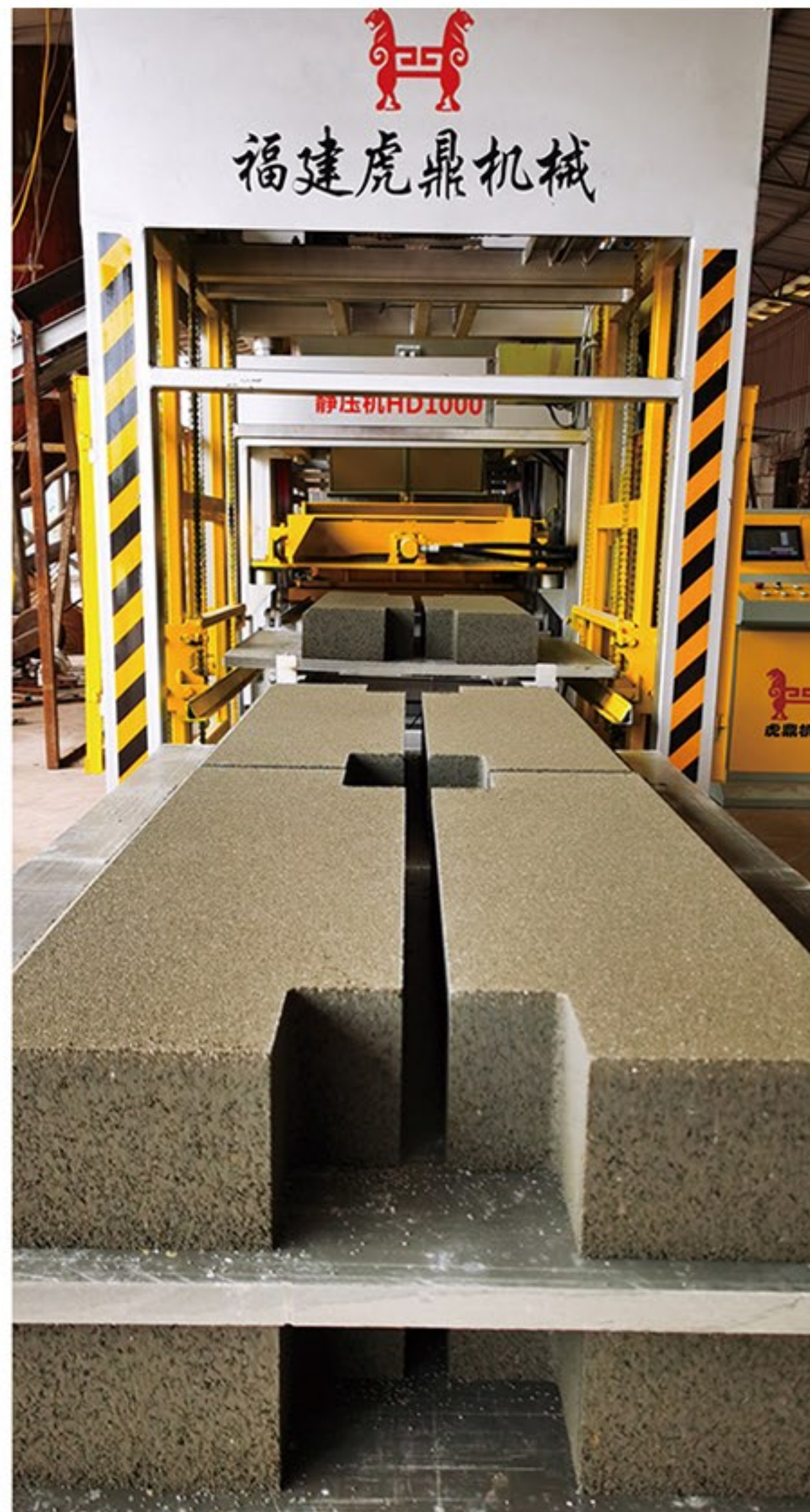
Production of kerbstones
